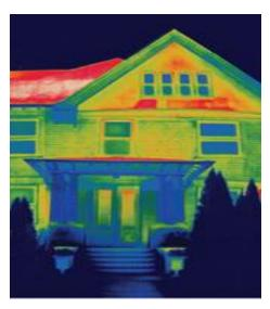
During an energy assessment, a Building Performance Institutecertified professional will use tools like a blower door test and infrared imaging (shown left) to figure out exactly where your home is losing energy and how you can fix these costly issues.
